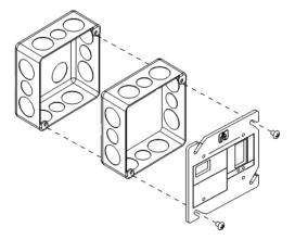
MOUNTS TO STANDARD 4"x4" ELECTRICAL JUNCTION BOX (EXTENSION RING INCLUDED—JUNCTION BOX NOT
